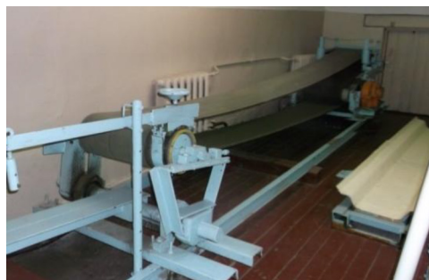
Fig. 1. Operational Model of a Horizontal Belt Conveyor ( \beta = 0 )
