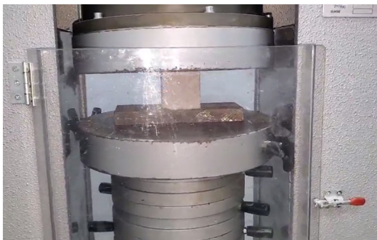
Fig. 4. Visualization of the process of testing formed limestone samples on the KL 200/CE-Tecnotest press
