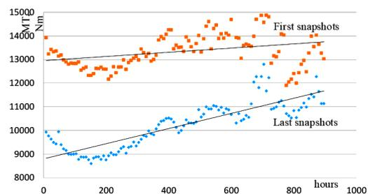
Fig. 4. Changes in the mean value of the motor torque (MT) in time at the beginning of the day and the end of the day of the experiment
