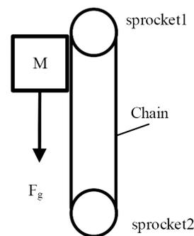
Fig. 6. Conversion of the chain friction force through the gravitational force of load with weight  $M$
