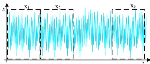
Fig. 2. The process of dividing the measured parameter ‘motor torque’ into frames
