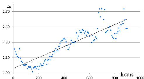
Fig. 7. Chain friction coefficient change in 912 hours
