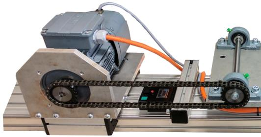
Fig. 1. Bench for research on the roller plate chain
