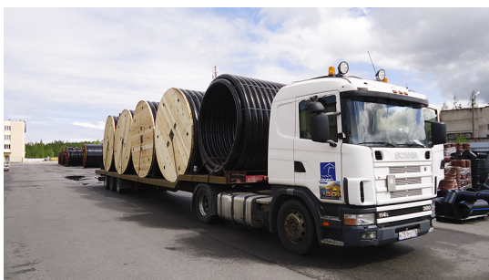
Fig. 4. Transportation of composite pipes in coils
