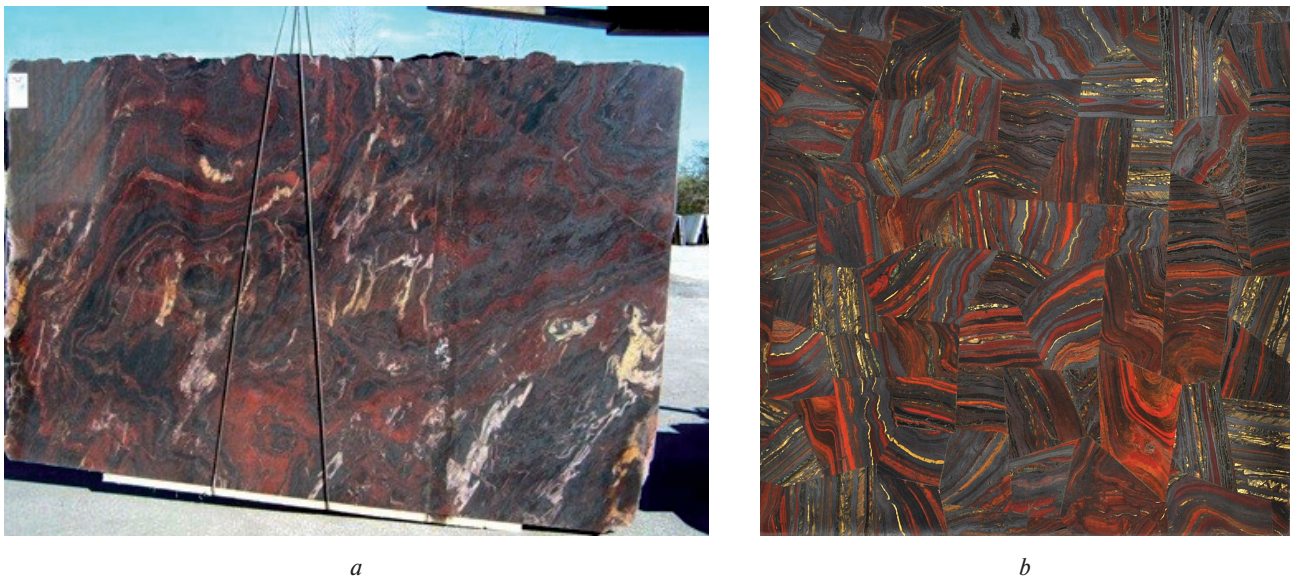
Fig. 4. Jaspilite slab (a), iron red granite, and standard plane (b) with dimensions of 30.5 \times 30.5 \times 1 cm, produced by "gem surface" technology [9]
