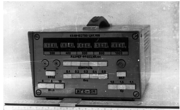
Fig. 2. The IGS-5M device for rapid measurement of the rock mass particle size distribution
