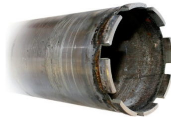
Fig. 2. The kind of the pilot drill bit with erosive track on the matrix
