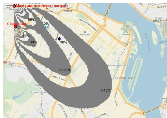
Fig. 3. Zone of pollution by sulfur dioxide with the direction of the wind from the northwest \alpha = 20^\circ , two sources of pollution
