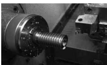
Fig. 2. The Worm Processing in the CN Lathes
