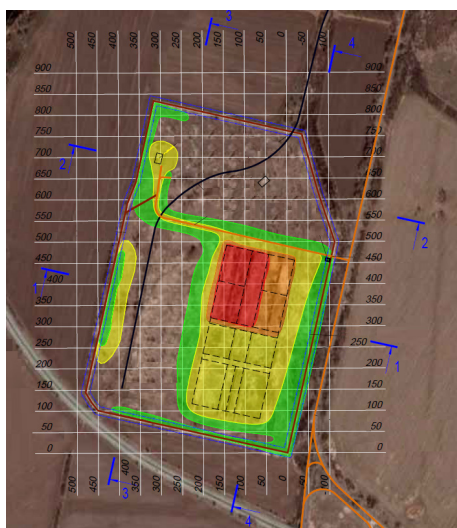
Fig. 5. Modifications of modeling the situation in 2015 at the “Base-S” industrial site for the research in the period from 2012 to 2019 (RRP measurement interval = 0 meters) and construction of 2-D model map with a grid size of 50 \times 50 meters
