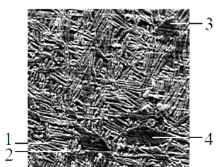
Fig. 9. Bronze with K_R = 0.35 ( \times 2,000 ) scanning electron microscopy image and X-ray spectral microstructural analysis results (Table) with local concentrations quantitate data
