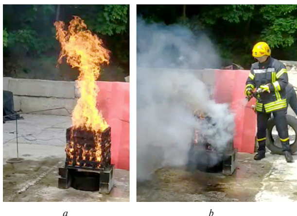
Fig. 6. The procedure for conducting the tests (model fire with pine beams) includes the following stages: a – free development of the fire; b – the process of extinguishing the fire
