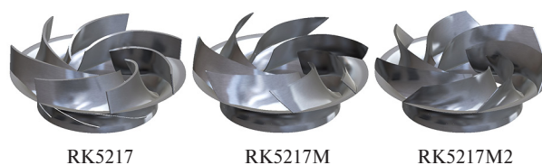
Fig. 2. Computer models of the blades of the investigated runners
