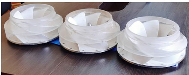
Fig. 3. Photo of three 5217 series runners (from left to right: RK5217M, RK5217, RK5217M2)
