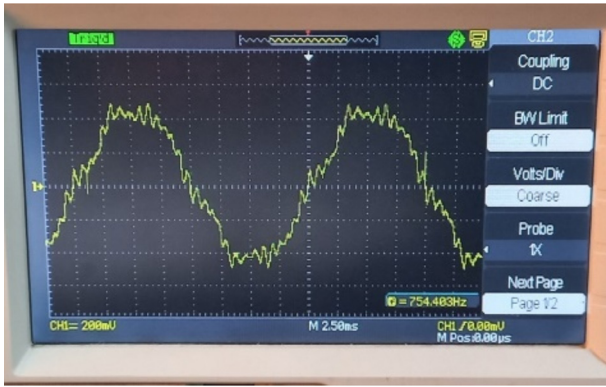
Fig. 13. Current characteristics of the LSPMSM on the oscilloscope
