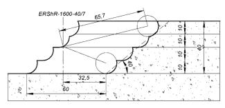
Fig. 2. Mine face profile of the excavator ERShR-1600-40/7 when working out the overburden bench with a height of 40 m
