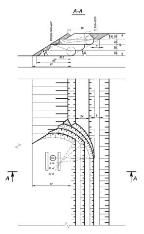
Fig. 3. Technological diagram of the ERShR-1600-40/70 operation during the development of an overburden bench with a height of 40 m with a forward trench
