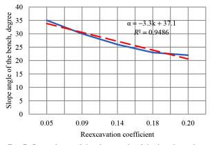
*Fig. 7. Dependence of the slope angle of the bench on the reexcavation coefficient*
