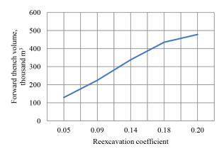
Fig. 6. Dependence of the forward trench volume on the re-excavation coefficient
