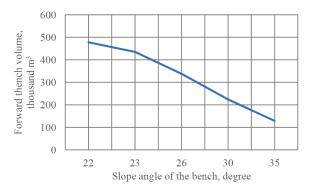
Fig. 5. Dependence of the forward trench volume on the slope angle of the bench
