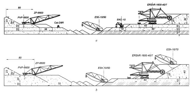
Fig. 4. Mining system of Pit No. 7 "Pivnich": a – the existing haulage mining system; b – the proposed combined mining system
