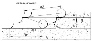
Fig. 1. Excavator mining face profile ERShR-1600-40/7 when working out the overburden bench with a height of 30 m
