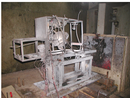
Fig. 3. Stand with a model engine installation after the accident
