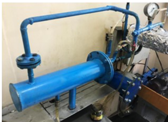
Fig. 5. Scheme (a) and general (b) view of the installation for obtaining low-boiling oil components by the analogy with industrial equipment
