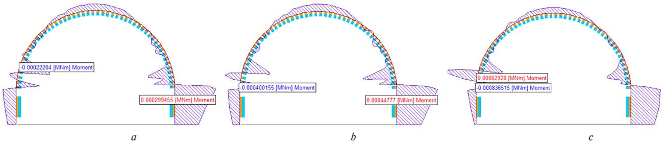
Fig. 8. Bending moments in the elements of steel arch made of SVP27:
