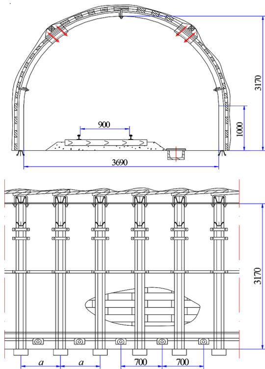
Fig. 9. SVP-22 steel arch support passport with steel arch distance 0.7 m (one-lane railway roadway)
