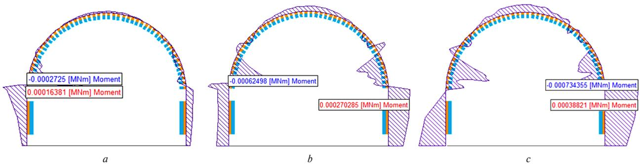
Fig. 6. Bending moments in the elements of steel arch made of SVP22:
