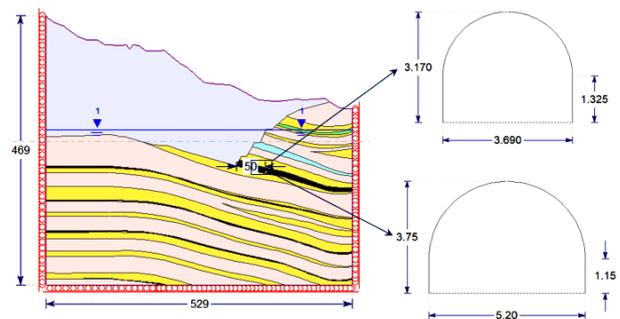
Fig. 4. Location and size of roadway in the numerical model
