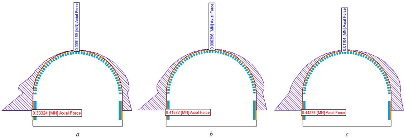
Fig. 5. Axial forces in the elements of steel arch made of SVP22:
