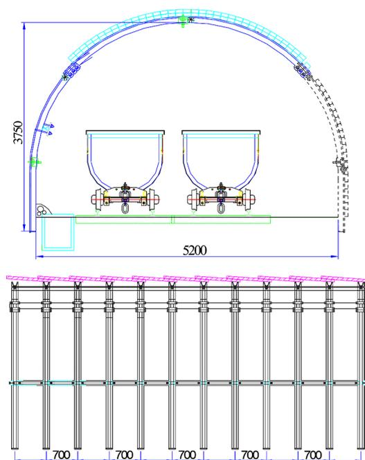
Fig. 10. SVP-27 steel arch support passport with steel arch distance 0.7 m (two-lane railway roadway)
