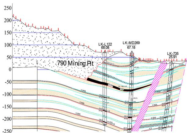
Fig. 2. The typical geological cross-section of the 790 open-pit mine filled with waste rock
