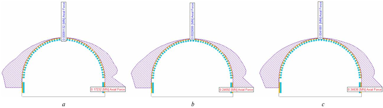
Fig. 7. Axial forces in the elements of steel arch made of SVP27:
