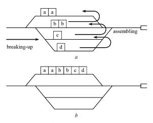
Fig. 3. Formation of a group train under conditions when one track is allocated for the accumulation of its cars: a – accumulation and assembling of cars; b – formed train
