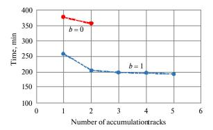
Fig. 4. The relationship between the time expenditures on shunting work, on the one hand, and the type of the trains dispatched, as well as the number of tracks allocated for their accumulation
