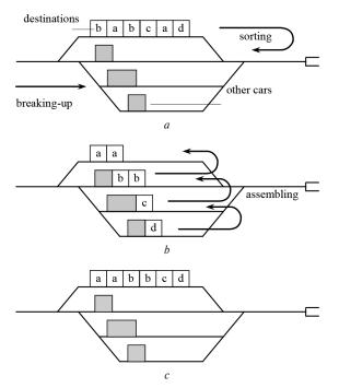
Fig. 2. Formation of a group train under conditions when one track is allocated for the accumulation of its cars:
