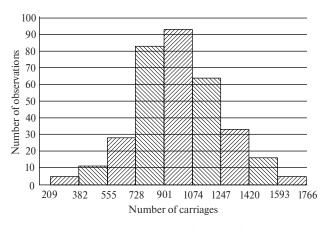
Fig. 1. Histogram and distribution function of a random value of the number of carriages entering the siding of LLC Transinvestservice during the day
