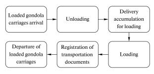
Fig. 2. The procedure for performing operations carriages, incorporated in the technological processes of metallurgical enterprises during the design
