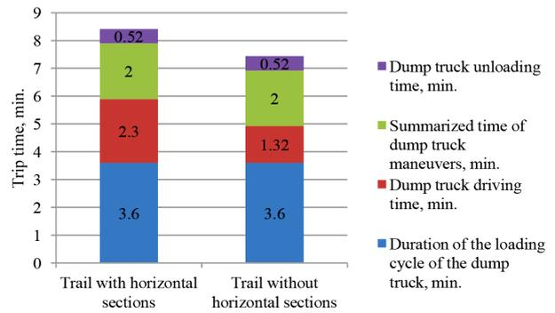
Fig. 4. Dependence of the dump truck trip time by component operations on the use of the existing and proposed schemes
