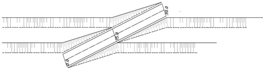
Fig. 2. Scheme of exit trails of auto transport without horizontal sections
