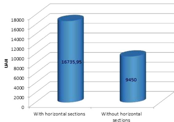
Fig. 5. Operating costs for maintenance and repair of open mine roads
