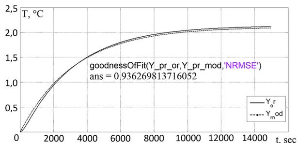
Fig. 5. Graphs of temperature time changes in the local indoor heating zone (solid line), and the model, determined with the use of identification of dynamic characteristics of a heating zone involving the proposed method (dotted line)
