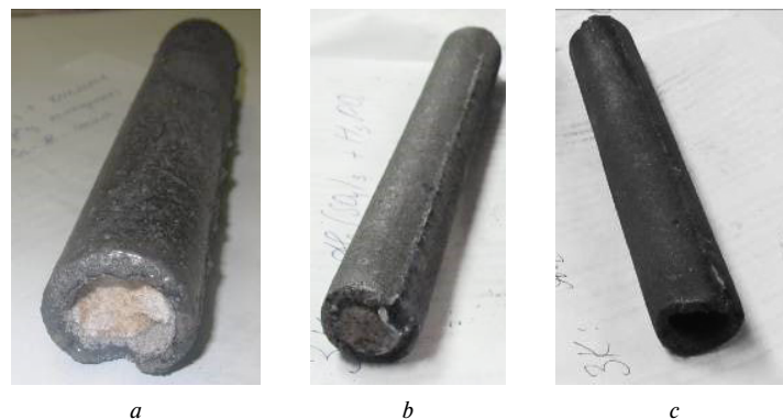
Fig. 9. Castings made using the developed core mixture:
