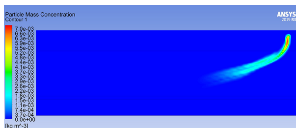
Fig. 13. Droplet concentration in the longitudinal section of the PRE zone
