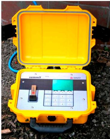
Fig. 2. Seismograph picture
