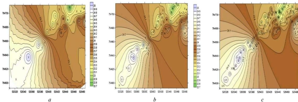
Fig. 3. Contour maps of geoid obtained from the Inverse Distance Model (Northern Zone): a – 25 – control points; b – 50 – control points; c – 100 – control points
