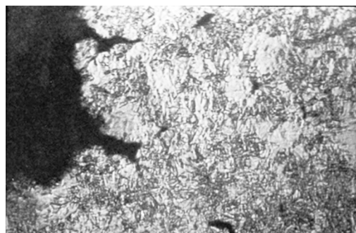
Fig. 4. Microstructure of deposited copper (longitudinal section), enlarged \times 120
