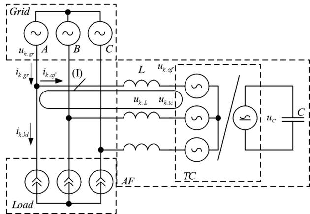
Fig. 1. Simplified equivalent circuit of the grid node with an active power filter
