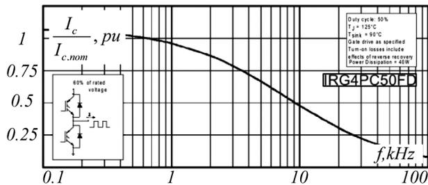
Fig. 6. The dependence of the collector current of the transistor switch IRG4PC50FD on the commutation frequency
