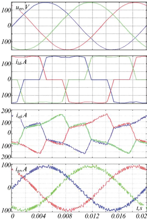
Fig. 2. Time diagrams of filter-compensating device in the system with a thyristor converter
