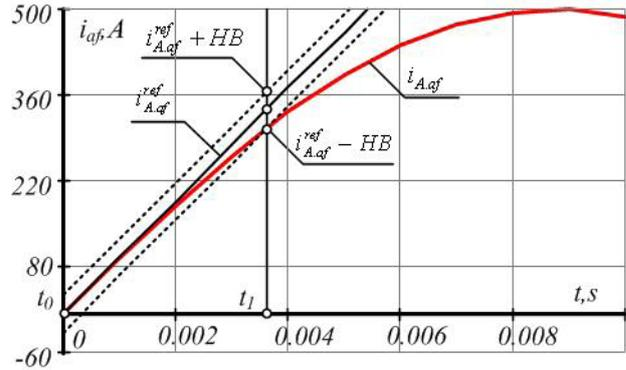
Fig. 5. Time dependence of transient current and determination of its deviations from the set value on the HB value
