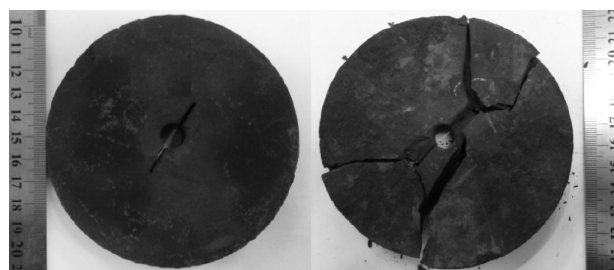
Fig. 2. The mode-II fracture toughness testing result obtained by Zhao Fei et al. in 2013
