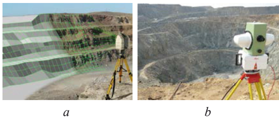
Fig. 1. Survey of near edge zone massif of a career with laser scanner Leica HDS4400
