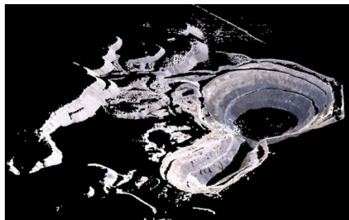
Fig. 8. Three-dimensional model of Vostochnyy quarry of Akzhal deposits
