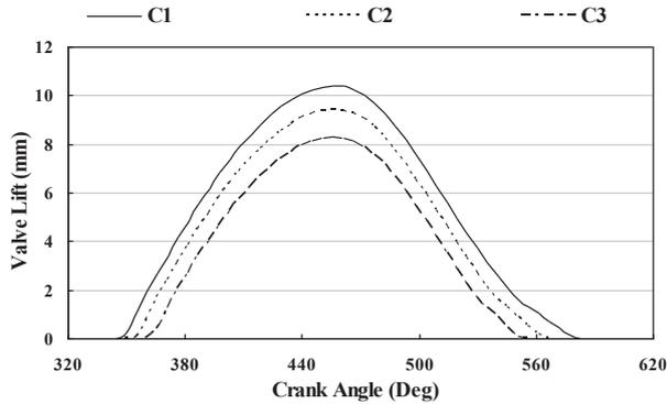
Fig. 4. The valve lift curves of different regulating quantity at 2000rpm
