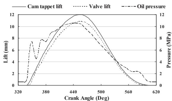
Fig. 3. The curves of cam tappet lift, valve lift and oil pressure at 2000rpm without regulating
