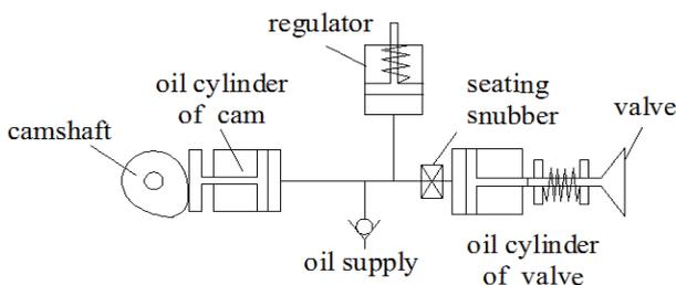
Fig. 1. Schematic diagram of hydraulic variable valve timing and lift system
