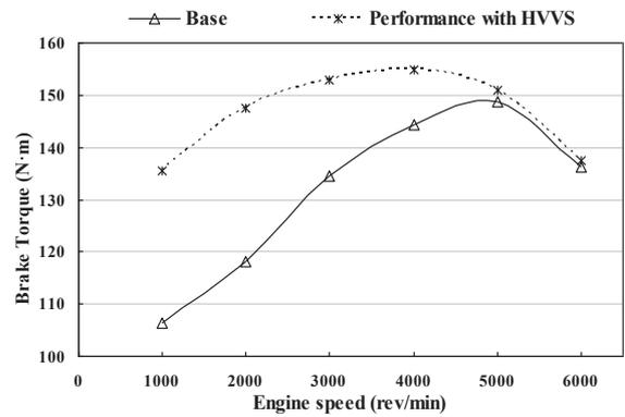
Fig. 11. Brake Torque versus engine speed of HVVS and base engine
