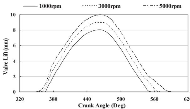
Fig. 6. The regulated valve lift curves for different speed
