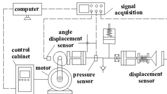
Fig. 2. Schematic diagram of HVVS test platform
