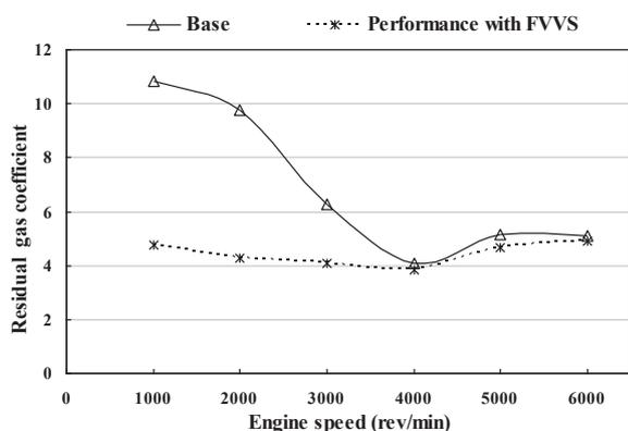
Fig. 13. Residual gas coefficient versus engine speed of HVVS and base engine
