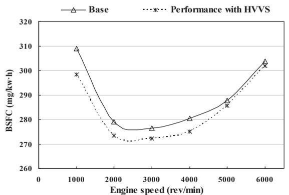
Fig. 12. BSFC versus engine speed of HVVS and base engine
