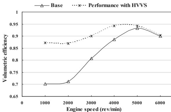
Fig. 9. Volumetric efficiency versus engine speed of HVVS and base engine
