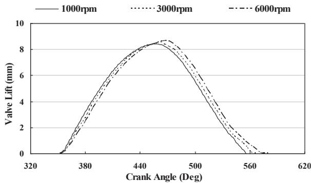
Fig. 5. The Valve lift curves with different speed under the same regulating quantity
