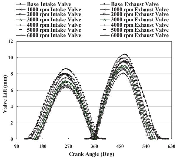
Fig. 8. Valve lift curves of HVVS and base engine
