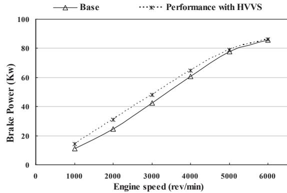
Fig. 10. Brake Power versus engine speed of HVVS and base engine
