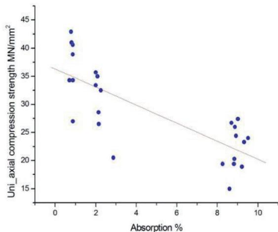
Fig. 7. Effect of absorption on uniaxial compressive strength
