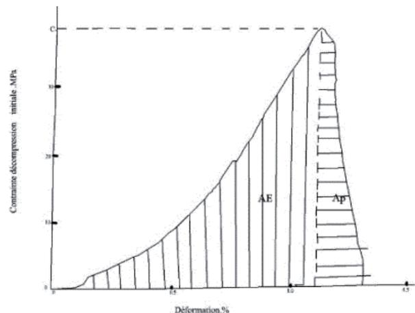
Fig. 4. The stress-strain curve after the peak stress was obtained for each curve by Tamaya Digital Planimeter measurements
