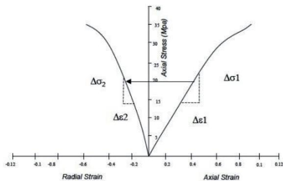
Fig. 6. Calculation of Poisson's ratio from stress-strain data:  $\sigma_f$  – axial stress;  $\Delta\epsilon_2$  – radial strain;  $\Delta\epsilon_1$  – axial strain;  $E$  – Young modulus
