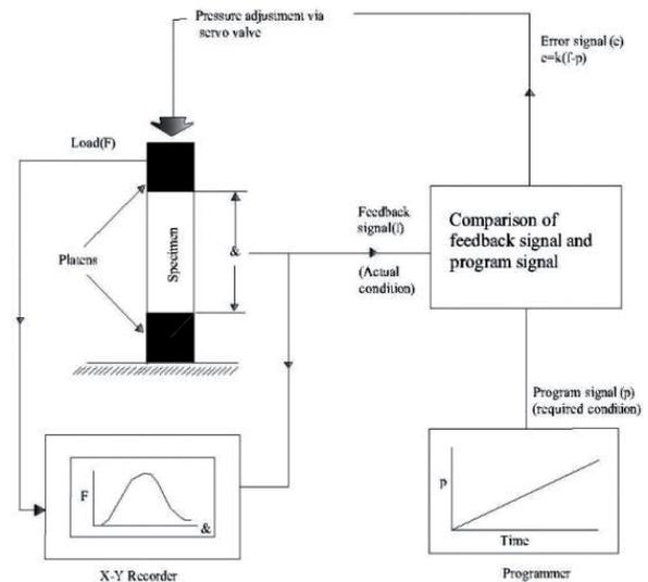
Fig. 3. Closed-loop programmable testing machine control system
