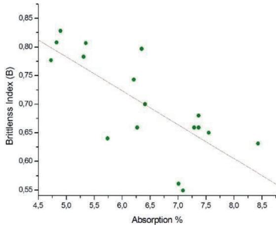
Fig. 9. Effect of absorption content on the brittleness index
