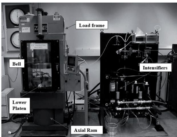
Fig. 2. Machine with tests servo controlled on the test sample
