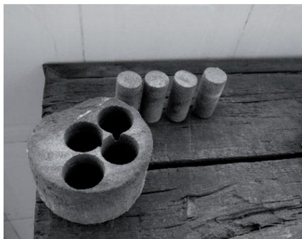
Fig. 1. Cylindrical sandstone specimen
