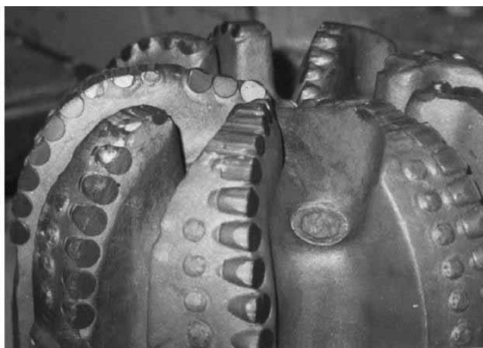
Fig. 5. Worn PDC cutters (drill bit-Read Hycalog 11 5/8 DS 66)
