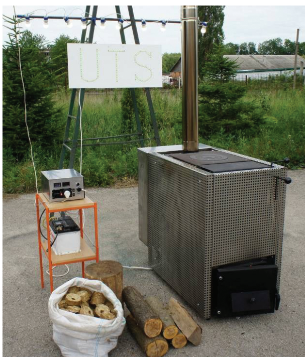
Fig. 6. Cogeneration installation that is based on a 20 kW heat generator with TEG block and modules of electric energy conversion and accumulation
