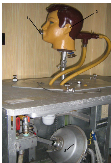
Fig. 3. A stand to determine half-mask resistance: 1 – sampling device from MIPRO undermask space; 2 – Sheffield dummy head; 3 – respiratory machine
