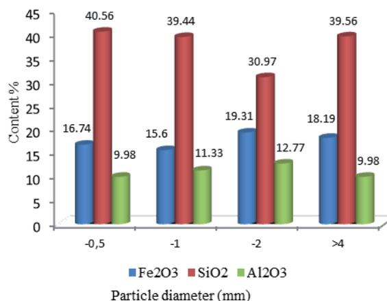
Fig. 13. Contents evolution of (Fe<sub>2</sub>O<sub>3</sub>, SiO<sub>2</sub> and Al<sub>2</sub>O<sub>3</sub>) in the sample washed with water (rejected) of Test n° 2
