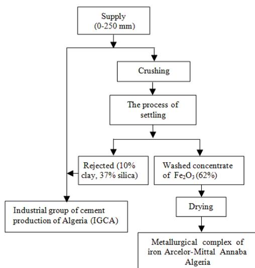
Fig. 16. Diagram of the proposed preparation for the enrichment of Anini's iron ore
