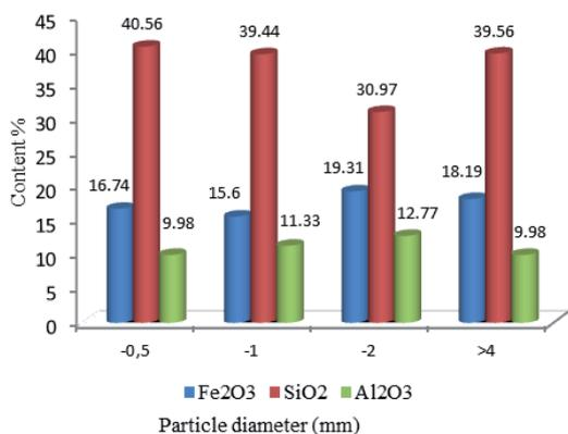
Fig. 11. Contents evolution of (Fe<sub>2</sub>O<sub>3</sub>, SiO<sub>2</sub> and Al<sub>2</sub>O<sub>3</sub>) in the sample washed with water (rejected) of Test n° 2
