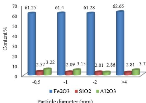
Fig. 10. Contents evolution of (Fe<sub>2</sub>O<sub>3</sub>, SiO<sub>2</sub> and Al<sub>2</sub>O<sub>3</sub>) in the sample washed with water (concentrate) of Test n° 1
