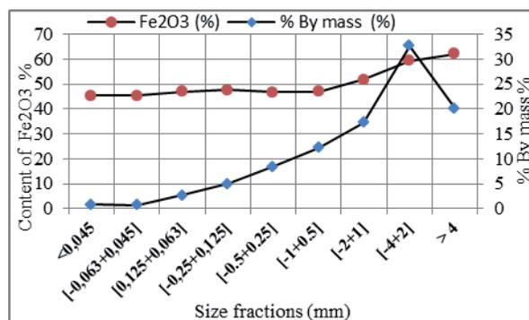
Fig. 1. Particlesize analysis of Anini iron ore
