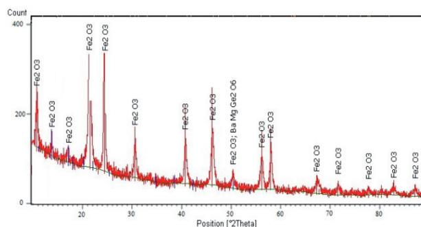
Fig. 14. Sample spectrum of the concentrate obtained after washing
