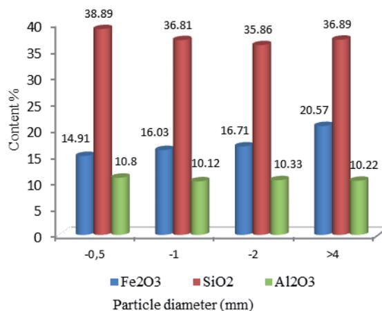
Fig. 12. Contents evolution of the (Fe<sub>2</sub>O<sub>3</sub>, SiO<sub>2</sub> and Al<sub>2</sub>O<sub>3</sub>) in the sample washed with water (rejected) of Test n° 1
