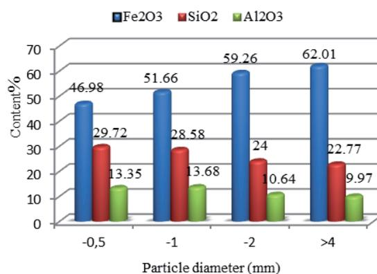
Fig. 2. Evolution of the levels of (Fe<sub>2</sub>O<sub>3</sub>, Al<sub>2</sub>O<sub>3</sub> and SiO<sub>2</sub>) of the studied iron ore
