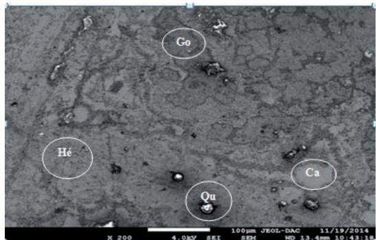
Fig. 8. Observation by scanning electron microscopy (SEM): He – Hematite; Go – goethite; Ca – calcite; Qa – quartz
