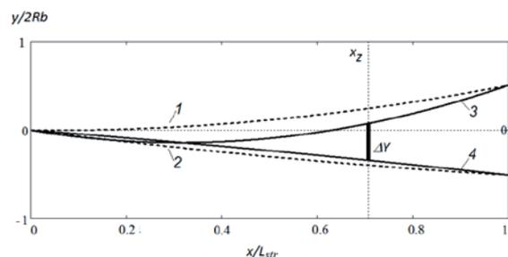
Fig. 8. Location of the string points corresponded to the maximum amplitude: 1, 2 – static sags of the upper and lower branches; 3 – the lowest coordinates of upper branch; 4 – the upmost coordinates of lower branch
