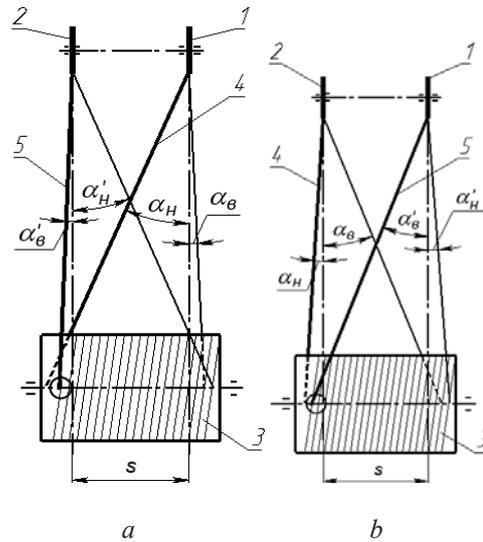
Fig. 1. The schemes of fastening ropes: *a* – standard; *b* – cross way; 1,2 – pulleys; 3 – drum; 4,5 – strings of ropes;  $\alpha_H$   $\alpha'_H$  – external deviation angles;  $\alpha_B$   $\alpha'_B$  – internal deviation angles
