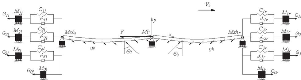
Fig. 6. Finite element model of a hoisting plant:  $M_{ib}$ ,  $C_{ib}$ ,  $a_{il}$  – parameters of  $i$ -th oscillator in the left branch;  $M_{ir}$ ,  $C_{ir}$ ,  $a_{ir}$  – parameters of  $i$ -th oscillator in the right;  $M_b$ ,  $M_{sh_l}$ ,  $M_{sh_r}$  – a drum mass, left and right pulleys;  $F$  – braking force;  $G_{il}$ ,  $G_{ir}$  – gravities in left and right branches
