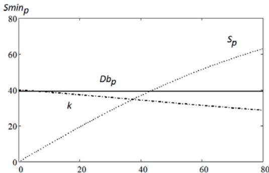
Fig. 4. Dependences of the reduced distance between strings on the dimensionless hoist parameters: 1 – drum diameter  $Db_p$ ; 2 – distance between pulleys  $s_p$ ; 3 – number of empty grooves  $k$
