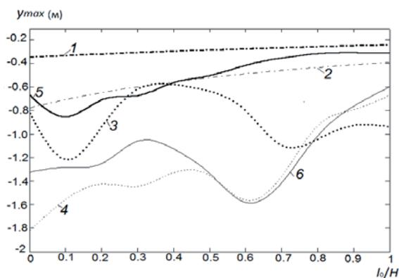
Fig. 7. The maximum amplitude dependences of the string mid-point sagging during transverse oscillations: 1, 2 – static string sagging in the branches with loaded and empty vessels; 3, 4 – maximum amplitude of oscillations in the branches with loaded and empty vessels during lifting; 5, 6 – maximum amplitude of oscillations in the branches with loaded and empty vessels during descending
