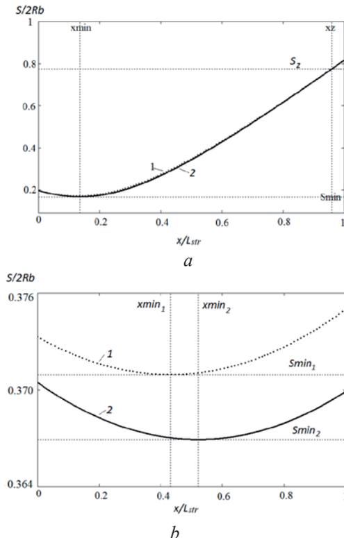
Fig. 3. The distance between branches: a – from pulley to drum; b – in the minimum value range; 1,2 – standard and cross ways of fastening
