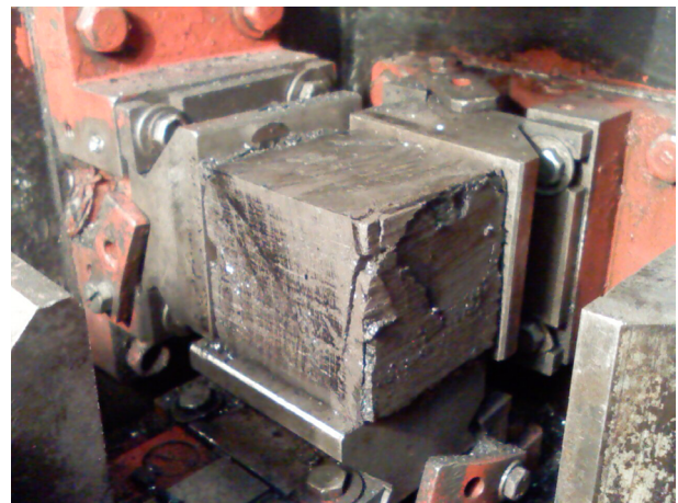
Fig. 1. The coal specimen in the chamber UCTC
